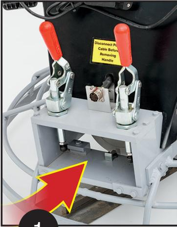
**1** With the troweler located in the work area, install handle.
