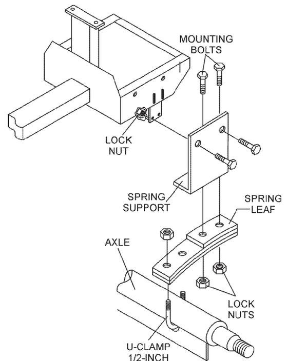
Figure 30. Suspension Components
