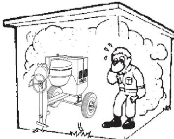
flow is restricted it will cause serious damage to the mixer or engine and may cause injury to people and property. Remember the mixer's engine (gasoline models only) gives off **DEADLY** gases.
