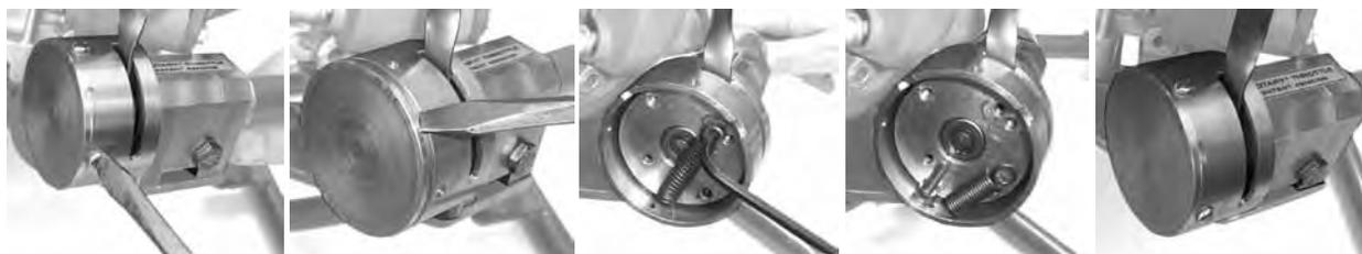
\* To return to **Idle/Maximum Speed** operation, the steps above must be reversed, applying Red Loctite™ (#271) to the screw to prevent it from getting loose during operation.
