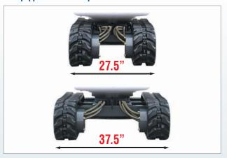
With the widest ranging expandable tracks in it's class, the 9VXE-3 can access tight spaces by retracting the tracks to 27.5" and expanding to 37.5" for greater stability and performance.
