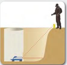
LINE SET: The Line Set/Check capability of the pipe laser allows you to raise the beam outside of the trench for fast line setup or checking. Raising the laser beam out of the trench to an above-ground stake saves you time—instead of having to move the excavator off line during setup of the pipe laser, you can just get on with your job. In addition, the Line Set-Check feature is ideal for rechecking the line in pipe jacking puts after each push. Only available on the DG711.
