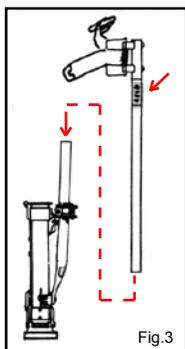
**Read the yellow label on the upper strut tube.** Keeping the strap buckles toward the toe of the stilt legs, slide the upper strut tubes down over the lower strut tubes and through the tube clamps. Position so the leg straps are just above the large portion of the leg calves. **Note: Do not bend or "size" the leg bands.** (Fig. 3-4)
