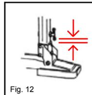
Set adjustable Dura-Stilts to the lowest setting and tighten wing-bolts well 1/4-1/2 turn past snug. (Fig. 12)
