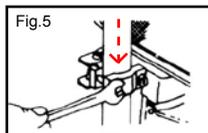
mered on or twisted harshly. Evenly tighten the two tube clamp bolts until the tube clamp just starts to grip the upper strut tube, then tighten each bolt an additional 1/4 turn. If strut tubes are secure, Stop! If additional clamping is needed, carefully tighten bolts 1/8 turn at a time until strut tubes are secure.
