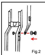
Attach lower strut tubes to the brackets or holes provided (identified by labels) with the attached 1/4 X 9/16 hex machine bolts and washers. Position washers on top of strut tubes under bolt heads. **Tighten well** when assembly is complete. (Fig. 2)
