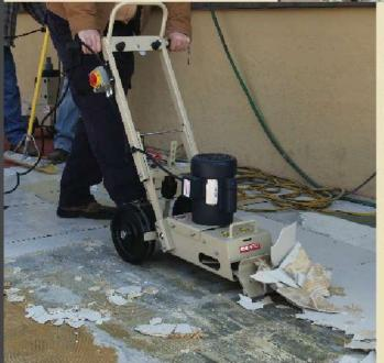
EDCO's TileShark™ Floor Stripper has an oscillating blade drive system that allows it to slice under the material making the removal easier and quicker.
