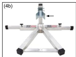
**Step 5.** Attach the cradle bracket (G) to the base (A) using the bolts (J), washers (K), and nuts (L). Secure with a 5mm hex key and 13mm wrench.
