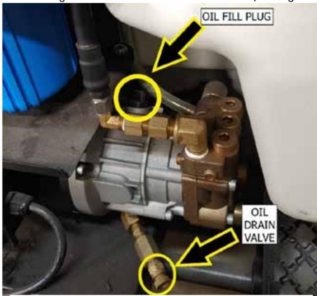
Figure 4 – Oil fill plug and drain valve location.
