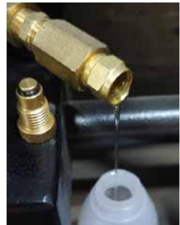
Figure 5 - Oil drain valve with end cap removed.
