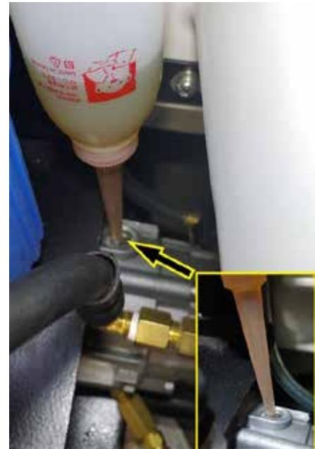
*Figure 8 – Vertical bottle orientation.*
