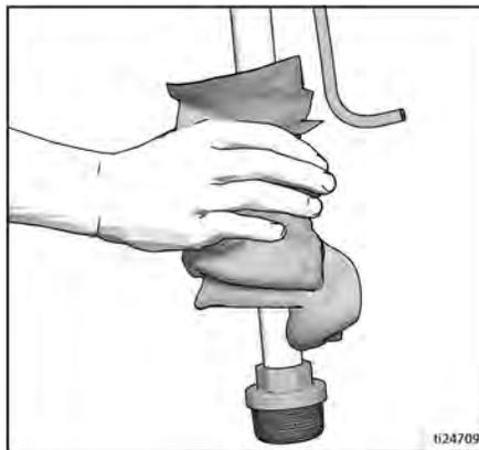
7. Place siphon tube set in grounded metal pail partially filled with flushing fluid. Use water for water-base paint and flammable materials for oil-based paint.
