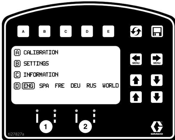
4. Press for Calibration. Set TRAVEL DIST to 25 ft (7.6m) or longer. Longer distances ensure better accuracy, depending on conditions.
