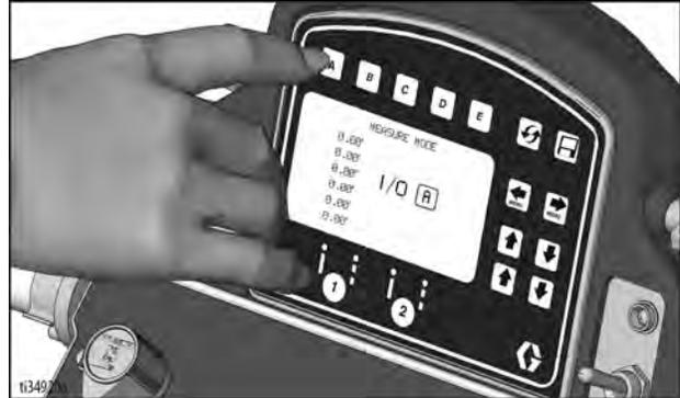
3. Press and release **A** to end measured length. Up to six lengths are viewable.
