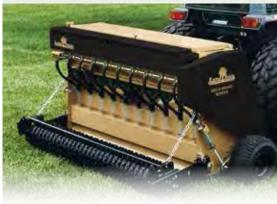
The optional small seeds box allows two seeds to be metered at one time into the same seed tube for even distribution.
