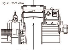
The post holes allow movement of the bridge +/- 0.5mm in either the left or right direction.
