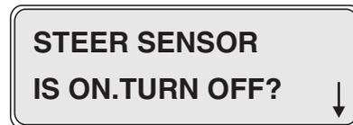
Note: Do not press the Enter button. Pressing the Enter button will disable the steer sensor
