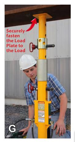
Screw the Release Knob shut on the Hydraulic Hand Pump, and begin pumping to raise the inner Lifting Tube and the Load.
