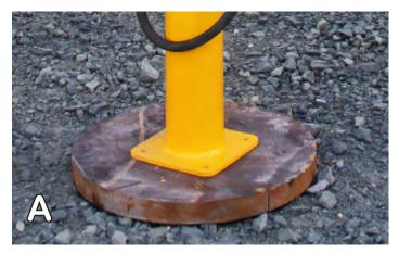
Put a secure base under the Post, one that will be able to fully support the load.
