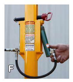
Slip both of the 5-ton Jack Cylinders, top first, into their welded Jack Pockets.
