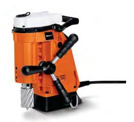
The Slugger JHM Magforce is a mag base drilling unit for diameters of up to 1 5/8" (40 mm). Designed for installation work, it features a quill feed enclosed in the housing. The motor and jig are cast from a single block.
