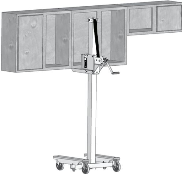
2. Operate the winch to raise cabinets into place. Lock the brakes on the casters and level the cabinets and fasten in place.
