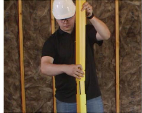
5. Fit the second boom section over the split boom connector. Align the corners access holes with those of the lower section.
