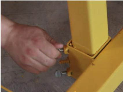
2. Tighten both lock screws on the dolly base to hold the boom tube securely.
