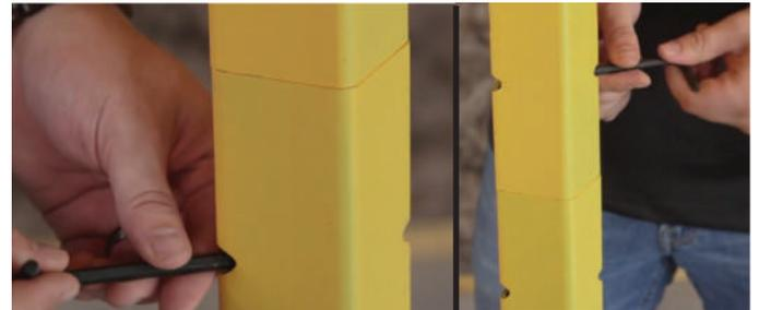
6. Using the hex key stored on the collar assembly, tighten both set screws on the split boom connector securely.
