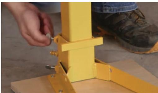
2. Tighten the thumb screws on the Counter Base to hold the Boom firmly in place. Install either of the boom sections into the Counter Base.
