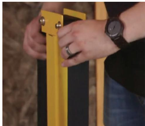
5. Position the strap over the top roller, making sure that it is aligned straight with no twists.
