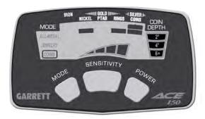
1. POWER Pushbutton (press and hold to reset to factory recommended settings)—Press and release to switch the unit ON and resume hunting with the same settings and modifications used prior to turning the unit OFF. When the POWER pushbutton is pressed and held for 5 to 10 seconds (until the detector beeps), the ACE 150 will return to the factory recommended settings of each MODE.
