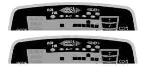
All Notch Discrimination modifications made while in the CUSTOM mode will be retained when the detector is turned OFF. However, all changes made to the Notch Discrimination scale while in the ALL-METAL, JEWELRY, RELICS
