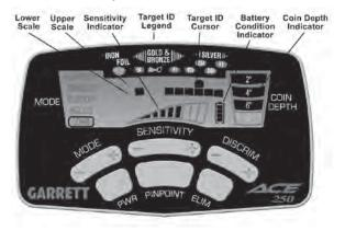
1. POWER Pushbutton (press and hold to reset to factory recommended settings)—Press and release to switch the unit ON and resume hunting with the same settings and modifications used prior to turning the unit OFF. When the POWER pushbutton is pressed and held for 5 to 10 seconds (until the detector beeps), the ACE 250 will return to the factory recommended settings of each MODE.
