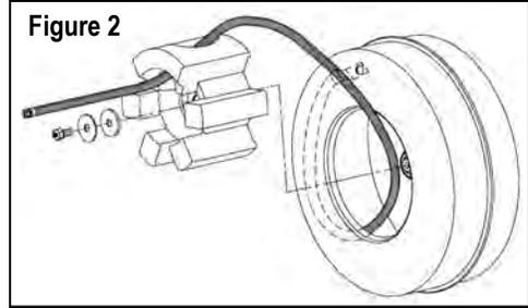
5. Slide the V-Belt (62") over the drum and hang it from the slip clutch. Push down on the motor enough to slide the V-Belt onto the drum.
