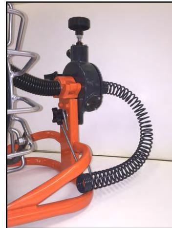
**THE CABLE AND SPRING ARE UNDER TENSION WHEN ATTACHED TO THE HOLDER. USE CAUTION WHEN RELEASING THE GUIDE TUBE FROM THE HOLDER.**
