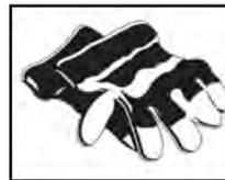
Only wear leather gloves. Never use any other type of glove, such as cloth, rubber, or coated gloves. Never grasp a rotating cable with a rag. These items could become wrapped around the cable and cause serious injury.
