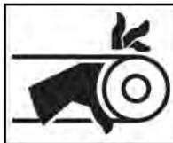
Never operate machine with belt guard removed. Fingers can get caught between belt and pulley.
