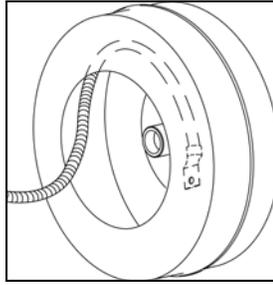
**Note:** The cable should lay in the drum in a clockwise direction.
