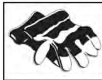
Only wear leather gloves. Never use any other type of glove, such as cloth, rubber, or coated gloves. Never grasp a rotating cable with a rag. These items could become wrapped around the cable and cause serious injury.
