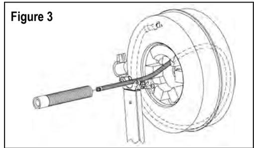
8. Then guide the knurled portion of the Flexitube spring into the front post clamp. (See photo)
