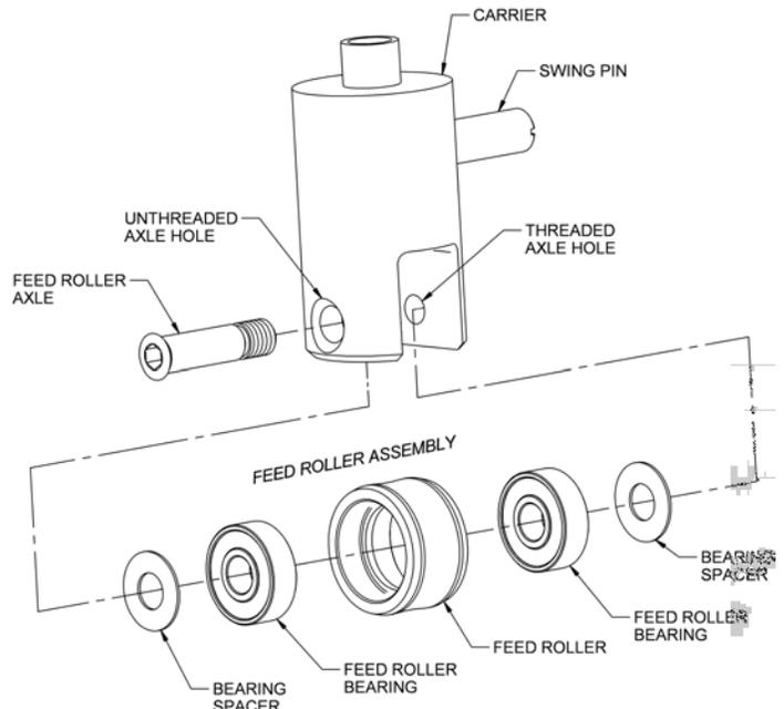
1. Remove the Feed Roller Assembly by unscrewing and removing the Feed Roller Axle.
