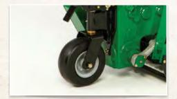
Semi-pneumatic swiveling rear wheel makes it easy to maneuver tightly around turns and cut closely along contoured landscape edges.
