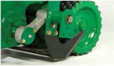
Easy depth and blade angle adjustment allow precise cutting in a wide variety of landscape contours and soil conditions.
