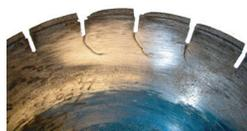
**Cracked Segments and/or Core:**
