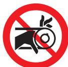
This symbol means do not insert fingers/digits under any edge of the belt cover while the engine/motor on the machine is running because personal injury and loss of fingers/digits may result. (Black pictogram with red "No" symbol outline)
