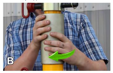
Screw the Threaded Locking Collar all the way down, to leave room for future adjustment.
