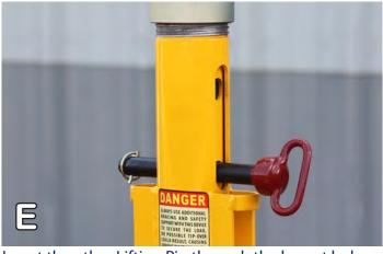
Insert the other Lifting Pin through the lowest hole possible in the Jacking Slot. Secure it with a Linchpin.
