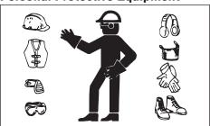
**Head protection** - must conform to ANSI Z89.1 and DO NOT wear under chin strapping while operating or within the operation area of the Horizontal Grinder.
