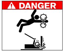
Support the equipment properly before you perform any work or maintenance beneath that equipment. Do not depend on
