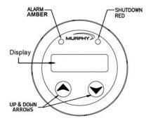
Access all menus and functions of the PV25 by using the **UP** and **DOWN** arrows on the front of the gauge. When power is first applied to the PV25, **Parameter** readings begin to display.
