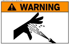
Check lines, tubes and hoses carefully. Do not use your bare hand to check for leaks. Use a board or cardboard to check for leaks. Tighten all connections to the recommended torque. Replace the parts if any of the following conditions are present:
