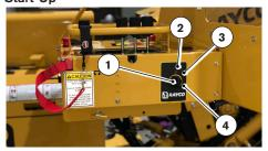
Insert the key (1), and turn the ignition switch to the Run Position (3) position for 10 seconds.
