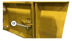
To swing the blade wings inward, pull the clevis pins (17) located on the back side of the blade. Simply turn the wings inward, reinstall the clevis pins at holes (18) located on top
