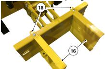
The RG55 comes equipped with a 50 1/2" wide blade. For convenience of trasporting through gates, or to load and unload on and off a trailor, the blade has wings (16) that can swing in to be only 34 1/2" wide.
