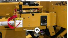
To adjust the command cut speed when using a RG55, adjust the needle valve (15) below the operator panel. If the cutter boom lunges while cutting the stump the command cut is set too slow. If machine stalls or is too agressive command cut is set too fast. Additional adjustments can be made while cutting the stump.
