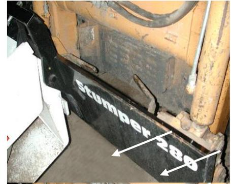
3. Hook up hydraulic hoses. NOTE: Be sure to run hydraulic hoses through the inside of bracket as shown.
