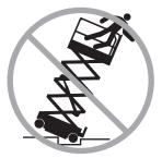
Do not operate the machine in strong or gusty winds. Do not increase the surface area of the platform or the load. Increasing the area exposed to the wind will decrease machine stability.
