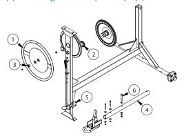
2) Assemble the chassi motor support (1) on lower column (2), fasten with the hexagonal bolt  $3/8"x\ 1"$  (3). Then, fasten the lower guide (4) and larger guide (5) on the chassi motor support (1) with hexagonal bolt  $3/8"x\ 1"$  (3). Fasten the motor support (6) on guides with hexagonal bolt  $3/8"x\ 2"$  (7).
