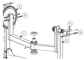
4) Position the steel yoke (1) in  $30^\circ$  angle. Place the drum (2) on the steel yoke (1) and tightening the hexagonal bolt 7/8''x2.1/4'' (3).
