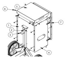
**6)** Fit pulley (1) on the pinion shaft (2), securing with retaining ring E-20 (3) and key 6x6x30.
