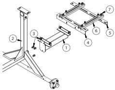
3) Assemble the steel yoke (1) on reducer (2) with hexagonal bolt 3/8"x4.1/2" (3). Assemble the bearing support (4) on the steel yoke (1) and fasten on the lower column (5) with bolt 3/8"x 3.1/2" (6).
