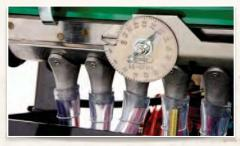
The seed depth guide allows for seeding at variable rates and for different grass varieties and applications.
