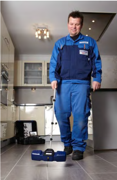
Fig. 13: Localizing the camera head underground
