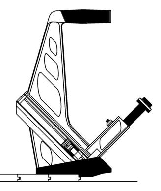
This improved version of our popular hardwood flooring nailer model H330 has been specially developed to address the need of the professional as well as the DIY or novice floor installer. Its ratcheted design allows the user to strike the nailer as many times as necessary to countersink the cleat. Hold the nailer in position until the plunger returns to its up position; then move it to the next location. It's that easy!
