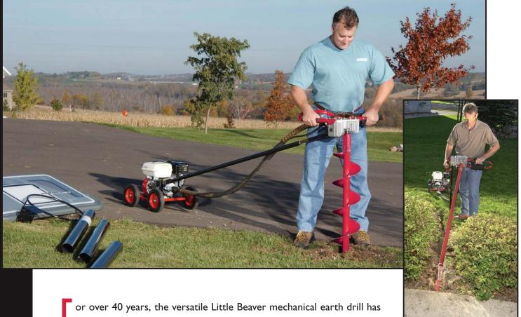
or over 40 years, the versatile Little Beaver mechanical earth drill has been the #1 choice of rental store owners, fencing contractors, and other professionals who require a one-man auger that is safe and simple to operate. Thanks to our patented torque tube, we've eliminated the kickback found in competitive augers, making one-man drilling safe and productive.
