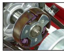
A reliable, centrifugal clutch slips when a buried object is encountered or the auger is overloaded. This protects the flexible drive cable and the transmission gears and shafts from damage.
