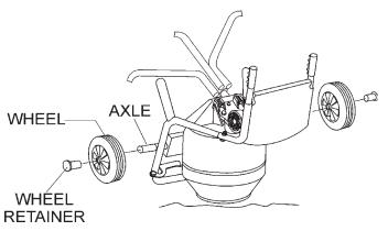
Figure 11. Wheels and Wheel Retainers
