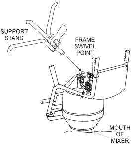
Figure 10. Attaching Support Stand
