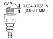
Figure 32. Spark Plug Gap
