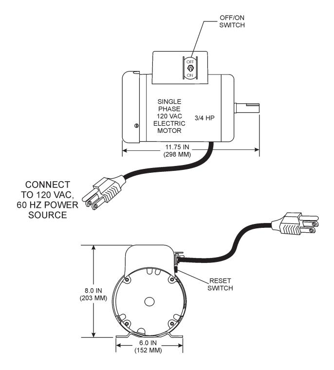
Figure 2. Electric Motor
