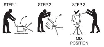
Figure 14. Tilting Mixer to Upright Position
