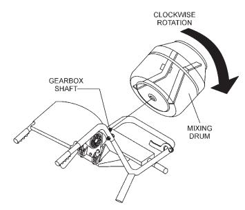
Figure 8. Mixing Drum Placement
