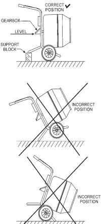
Figure 29. Mixer Positioning (Gearbox Oil Level)
