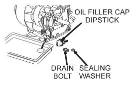
Figure 33. Engine Oil (Draining)
