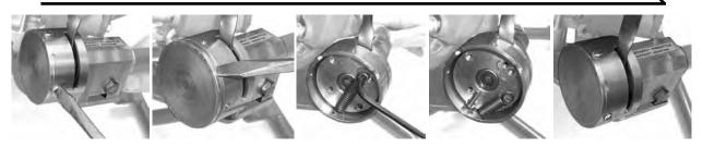
\* To return to **Idle/Maximum Speed** operation, the steps above must be reversed, applying Red Loctite<sup>™</sup> (#271) to the screw to prevent it from getting loose during operation.
