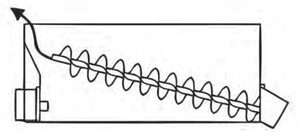
STEP 7: Place the auger on a secure work platform. Use a hammer and chisel to remove the lock nuts from the flights to be replaced.
