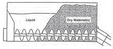
STEP 2: Run the auger in reverse. This will draw the dry material(s) into the liquid and up the motor end of the bucket. The mixture will roll back into the mixing material.
