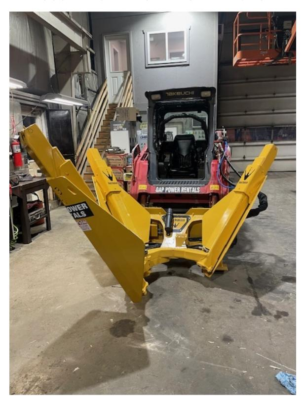
There is a harness and controller in the cab needed to operate the spade. Whenever we send it out on our machine we need to install it properly. If it goes on a customers machine we should be advising him how to run the harness.
