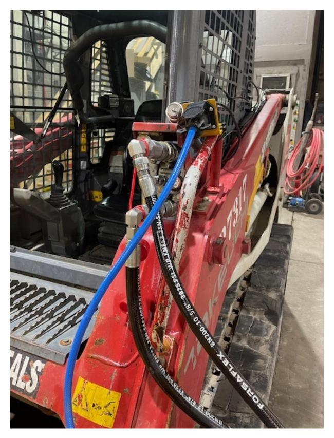
Zip tie the plug somewhere around the quick coupler. Run the wire down the boom arm zip tying it in place along the way. Once it reaches the back of the boom arm turn and route it along the cab and then into the window. Please take care to do this step well to prevent damage to the wiring! There are 11 wires in the loom!
