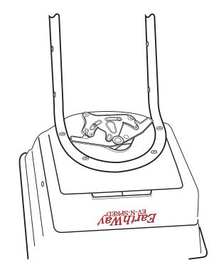
**4.** Install Gearbox by inserting the pinion shaft into hole in center of hoppers bottom. The word **"FRONT"** on the gearbox must point to **FRONT** of the hopper.
