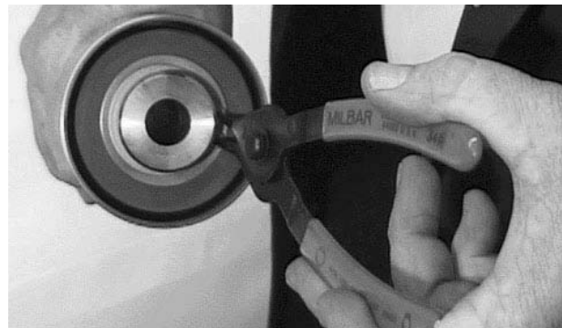
Figure 8-15. Remove Retaining Ring with Retaining Ring Pliers.
