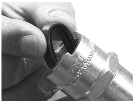
Figure 8-9. Remove Gasket from Coupling Socket.
