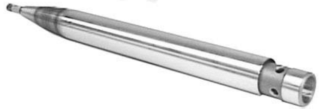
Figure 9-22. Slide Striker into Body/Anvil.
