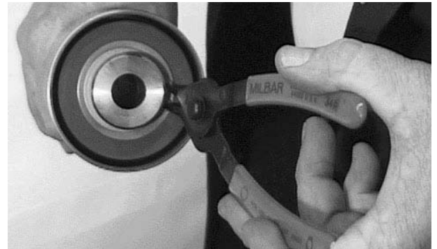
Figure 9-13. Install Retaining Ring with Retaining Ring Pliers
