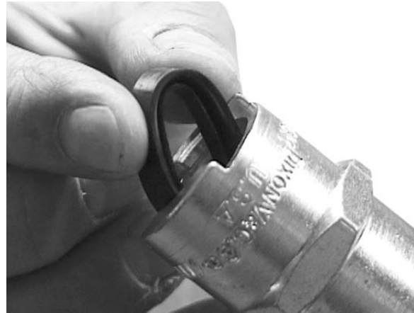
Figure 11-3. Install New Whip Hose Assembly
