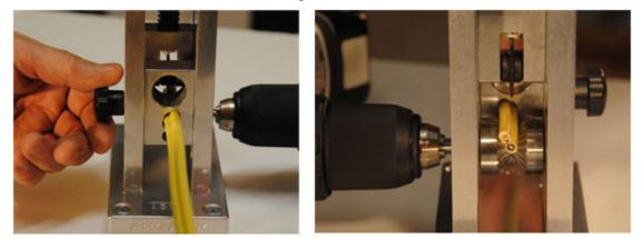
5. Lower the Knife Blade to touch the insulation/plastic, move the Front Wire guide down so the wire feeds in an 10-20 deg. angle
