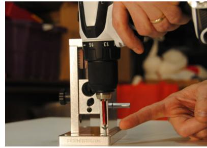
1. Secure the StripMeister<sup>TM</sup> to your workbench using the screws supplied thru the mounting holes
