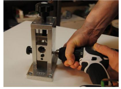
3. Loosen the front wire guide to enable the wire to hit the Feeder Drive v-groove
