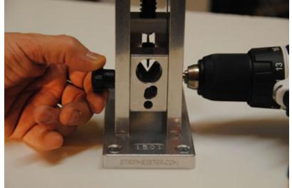
4. Place the wire through the wire guide onto the Feeder Drive vgroove
