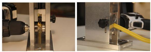
6. Tighten adjustment knob for front wire guide on the left side
