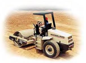
cohesive soils. The lightweight, single-piece engine enclosure is hinged at the rear to allow unobstructed access to the engine, radiator, battery, filters and daily maintenance checkpoints.
