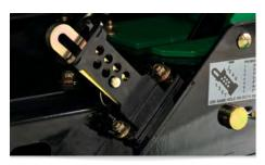
Aeration Depth Control for precision aeration in varying soil conditions; aerates up to 5" deep, in half inch increments.
