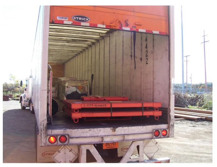
As you can see, the Basic 3 is an extremely lightweight box; in fact it is only slightly heavier than it's aluminum counterparts at a fraction of the cost. Depending on the size, some of the B3 models are capable of reaching depths up to 24' in C soil.
