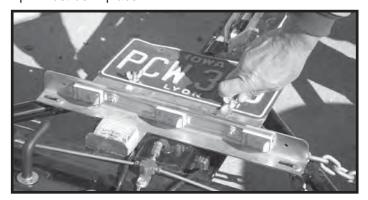
**Step 3.** Loosen wing nut on back of license plate holder, turn the clip on the front to a horizontal position and put license in the "down" position. Turn the clip back so it rests against the back of the light bar to hold the license down and tighten wing nut.
