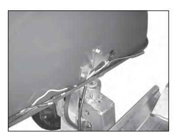
2. Cut nylon wire tie from wiring to brake hose on main frame, (used for shipping purposes only). Fish the three wires from main unit through the hole in fender.
