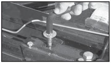
**Step 2.** Remove black locking pin **BEFORE** loading vehicle onto the Kar Kaddy. The removal of the locking pin allows "Auto Steer" to operate. When towing the dolly empty, this pin must be in place.
