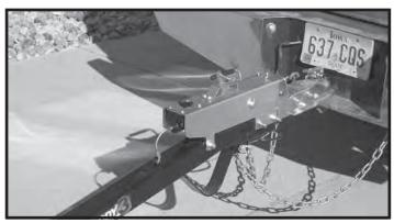
**Step 1.** Secure ball coupler to 2" (6,000 lb. capacity) towing vehicle ball only. Make sure that the hitch and the hitch ball are in good condition and not rusted, loose or stripped. **Recommended ball height is 18" to the top of the ball.** Make sure hitch is locked down and secured with safety clip. Criss-cross safety chains under tongue and secure to towing vehicle frame.
