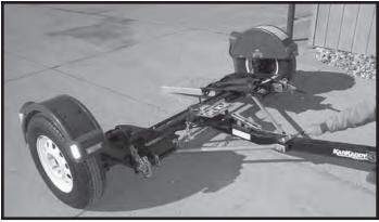
**Step 5.** Grasp bed release handle on tongue and pull toward coupler. This releases the tilt bed to permit loading.
