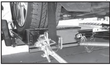
**Step 9**. Be sure tie-down winch is centered with the tire before tightening straps.
