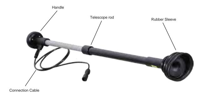
Due to the telescopic function, the sensor rod can be adapted to the user's individual height. The sensor rod is connected to the microphone connector on the right hand side of the device. The gas sensor is located at the bottom of the rod and covered by a rubber foot. Do not put the sensor under water.
