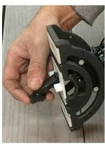
the top of the latch on the front of the tool, its above the tip. Holding the top of the latch pull out away from the tool, it is hinged. Rotate it down towards the tip, keeping the arched lower latch against the tip. Keep pushing down until the latch pushes the tip free from the lower housing of the tool. The tip will only come out through the base, at the hole in the gap spacer plate. Reinstall or install new tip in reverse steps.
