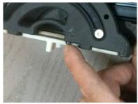
Slide the plate in, and the pin should drop back down by spring pressure. The pin will hold the gap plate in place while the tool is being used. Push the pin in, and slide the plate out when you wish to change plate gap size.
