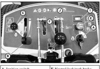
A. Ignition switchF. Neutral lock/park brake<br/>leverB. ThrottleI. Hour meterC. ChokeI. Hour meterE. Deck clutch switchJ. Oil pressure light (electric<br/>start only)
