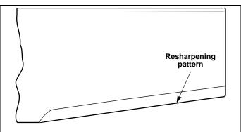
Do not sharpen to original pattern (below). It is easier to get a straight cutting edge following the resharpening pattern shown above.
