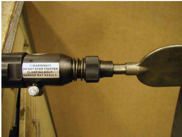
Pictured above shows the chisel installed. To remove a chisel reverse the above procedure and pull the chisel out of the chisel holder.
