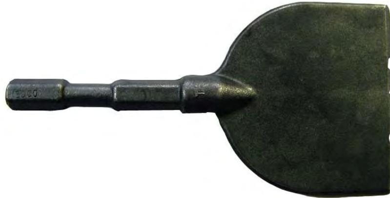
The above is an example of a chisel that has been abused, probably hitting inserts, studs or other objects embedded in the working surface. To get maximum life out of a chisel be careful when working around objects protruding out of the work surface.
