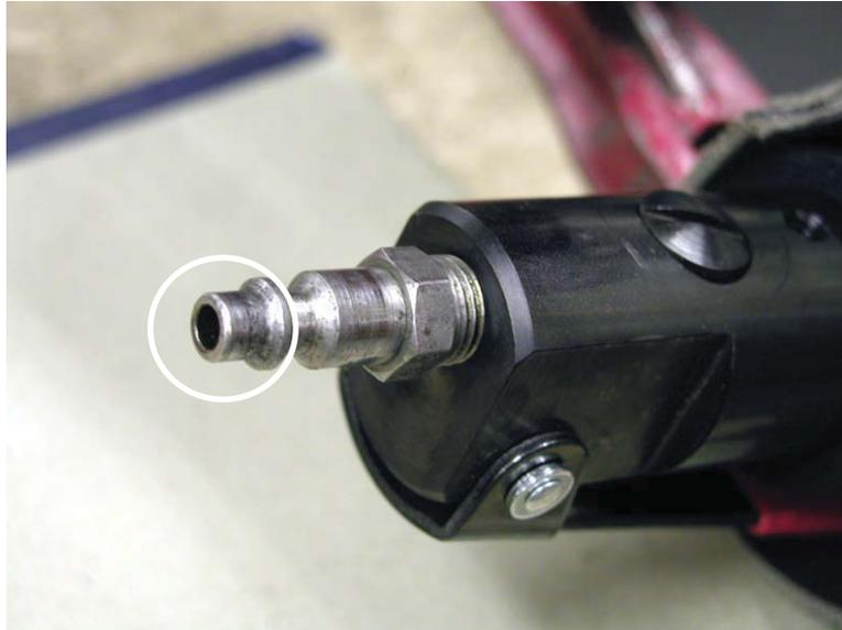
To lubricate the ALR put four (4) to five (5) drops of light weight machine oil in the hose connector circled above before connecting the air supply, graphite oil in extremely cold weather.
