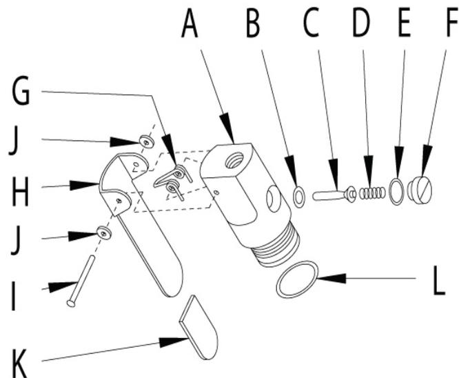
first remove the Capping screw (F). Note that the Valve Stem (C) should be replaced if it is worn and loose in Valve Body (A).
