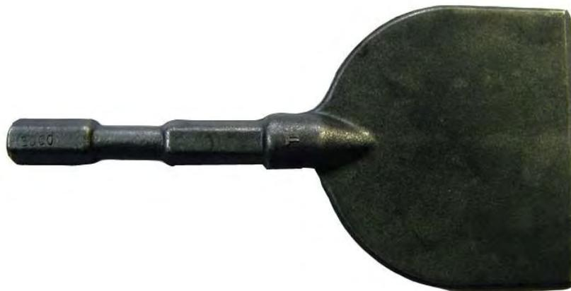
The above is an example of a chisel that has not been abused, as you can see the wear is *even* across the width of the chisel. Chisel edge may be renewed by grinding.
