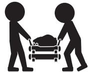
Do not turn the compressor over or lift it with a hook or rope.
