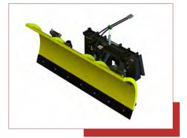
IMPORTANT: All replacement hydraulic hoses and fittings must have a minimum rated working pressure of 4000 psi. Hoses and hydraulic couplers from the attachment to the loader are included for skid-steer only.
