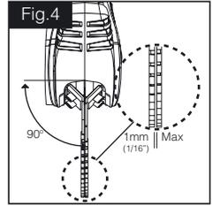
If the gap between the blades is too large, remove and gently bent inward to adjust the gap. Ensure that both blades are aligned vertically to the tool (See fig.4).
