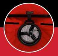
The Mini Fan Blower Door System uses the Duct Blaster fan and can be used to conduct blower door tests on small or tighter apartments and homes.
