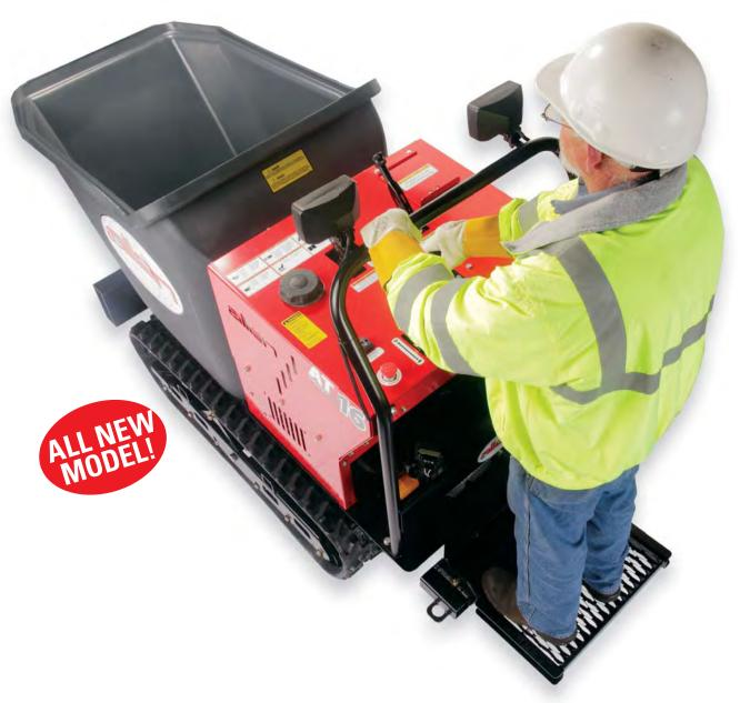
The **ALL-NEW** sixteen cubic foot AT16 Power Buggy with Track Drive provides excellent traction on grades, inclines, and soft soils. Providing more horsepower, more load carrying capacity and greater bucket volume than competitors; the new track buggy's rugged steel frame increases load weight and distributes the load across the entire frame, providing for smooth, even transport.
