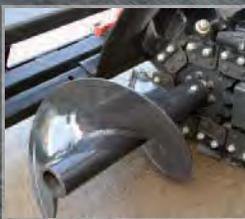
Replaceable spoil auger mounds most spoil to one side of trench.
