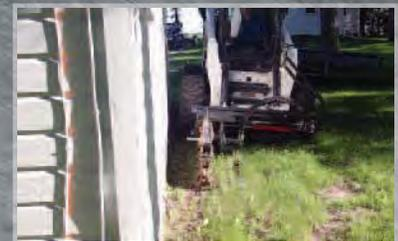
Side-shift allows for trenching closer to structures.
