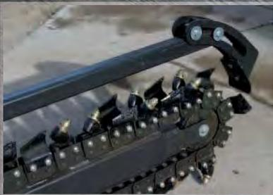
Built-in crumpler for loose soil removal.
