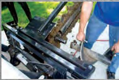
Auger is removable, allowing operator to trench close to obstacles when using side shift.
